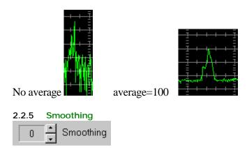
The smoothing function averages FFT bins within the same sample data block. This function is useful for wide bandwidth signals and smoothes the overall shape of a wide signal.
