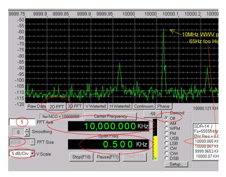
4. Stop the capturing and open the SDR-14 Setup menu. Notice the measured frequency has been automatically placed in the box(if you had peak markers checked and it was marking the correct reference peak) One can manually enter the Reference and Meas frequencies if not using a 10MHz reference.
