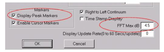
In the direct input mode, a value of 4.5dB will be very close since this is the level in dBm where the A/D begins to clip. If the internal preamp or an external one is used, then one must change the value accordingly.
