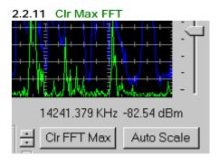
This button is used to reset the max hold buffer when the maximum hold display is active.
