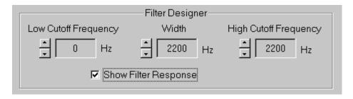
This menu allows the user to customize the demodulator filter width and positions. For single sideband modes (USB, LSB) the low and high cut positions can be adjusted independently. The other modes are symmetrical around the center frequency and so only the width may be adjusted. The filter alpha's are determined by the program and are not user definable.
