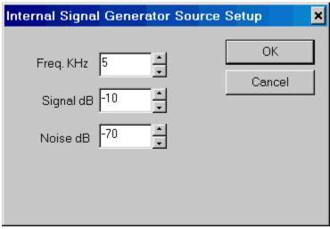
This menu is used to set the internal test generator signal amplitude, frequency and noise source levels. This is a simple real mode sine wave generator running at 48KHz with a Gaussian noise generator that can be added to the signal.
