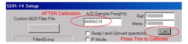
6. Go back to the main screen and start the captures again to verify that the new calibration has taken affect. One may have to perform this a few times to iterate the error to zero if the signal is noisy or the SDR-14 is still warming up.
