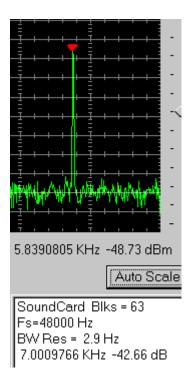
2. Left click on another part of the waveform and the first red marker freezes at the last value of the spectrum and a new yellow marker attaches to the new FFT position. It can also be moved with the function keys. The numeric value of the delta between the two markers is now shown in the INFO box.
