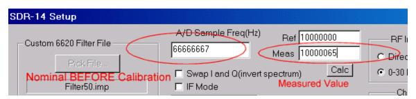
5.Click on the "Calc" button and the new A/D Sample Frequency is calculated. The "Meas" box will revert to the Ref frequency so one doesn't accidentally keep scaling the A/D sample frequency.
