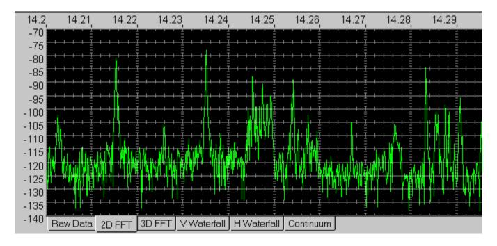
An alternative 2D view is available by choosing the "Color 2D Graph" selection in the FFT Setup Menu. This view adds color to the display in place of the internal scale markings. The colors correspond to the Waterfall color palette.
