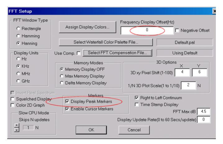
3. Setup the main screen as follows with an FFT size of 65536, an average of 5 or so, a center frequency of 10MHz(for WWV), demod OFF, and a span of 500Hz.. Press Start and adjust the screen to allow easy viewing of the 10MHz peak. Note the little blue x on the peak and its corresponding marker frequency of 10000.065Khz in the info box. This is the measured frequency of WWV and shows that the program is off by 65Hz.
