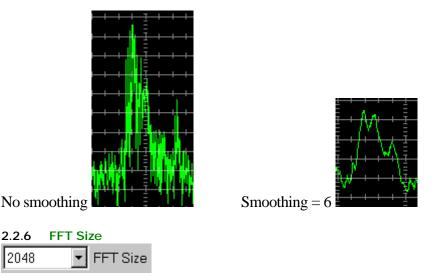
The FFT size pull down selection control is used to select the size of the FFT. The range is from 2048 to 262144 points. The larger the FFT the better the frequency resolution but the longer it will take to process since more data points are required between updates.
