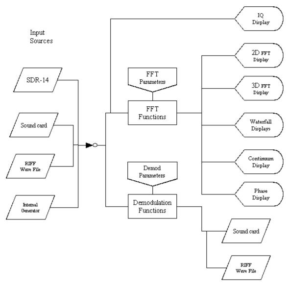
The data input can come from the USB port and an SDR-14 unit, a soundcard, a RIFF .wav file, or an internal test generator. A simple display of the raw data is available which is useful to set audio levels on a soundcard or adjust DC offsets.
