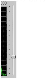
This control is used to move the viewable vertical window of the display. The control can be changed by dragging the control arrow or by clicking on either side of the arrow. The total range of the display is -140 to 140 dB referenced to full scale.
