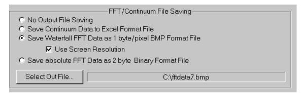
This menu specifies a 1 byte per pixel .BMP graphics file of the waterfall display to be written. If the "Use Screen Resolution box is checked, the image width will be the same as the screen pixel width. This mode creates images that are the same size as the program screen for easy viewing and reduced file size.
