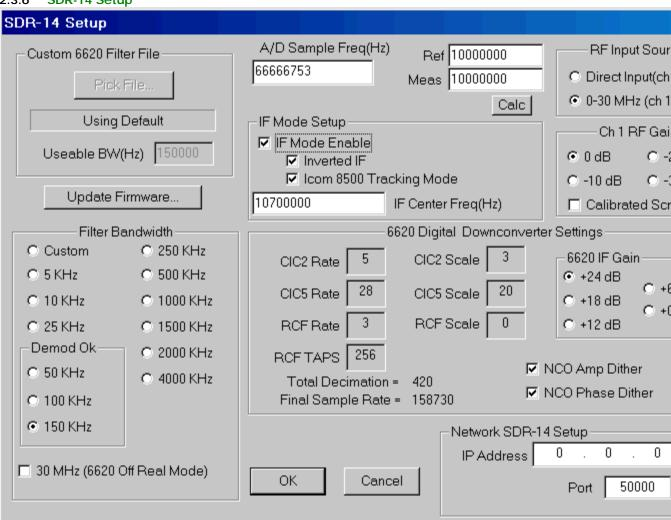
This setup menu is used to set the main parameters of the SDR -14 hardware.
