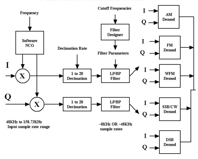
I/Q data from the input source is sent to the demodulator block. It is first "tuned" to the desired signal using a complex mixer and software NCO. This allows one to tune in signals anywhere within the input bandwidth which could be up to 150KHz wide..
