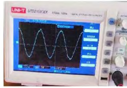
Fig. 6 Frequency waveform diagram of 1KHz Fig. 7 Frequency waveform diagram of 500Hz
