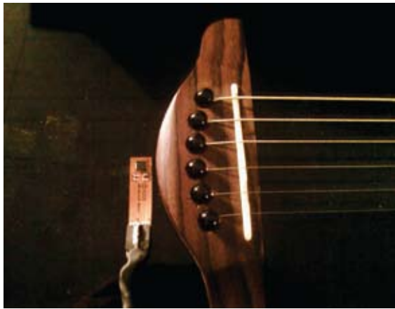
Figure 7. Accelerometer mounted on Fender Stratocoustic acoustic guitar.
